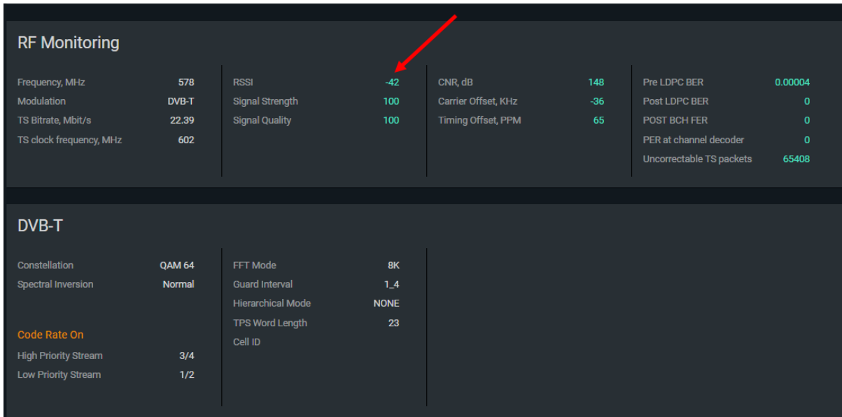
Figure 4 –Signal level in TS Analyzer interface
